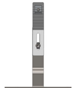
Tile Interface connection with elongated hole
